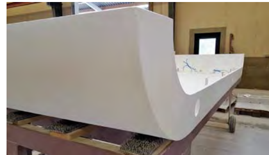
Figure 4: The typical thickness of GRC for façades is 12mm.
