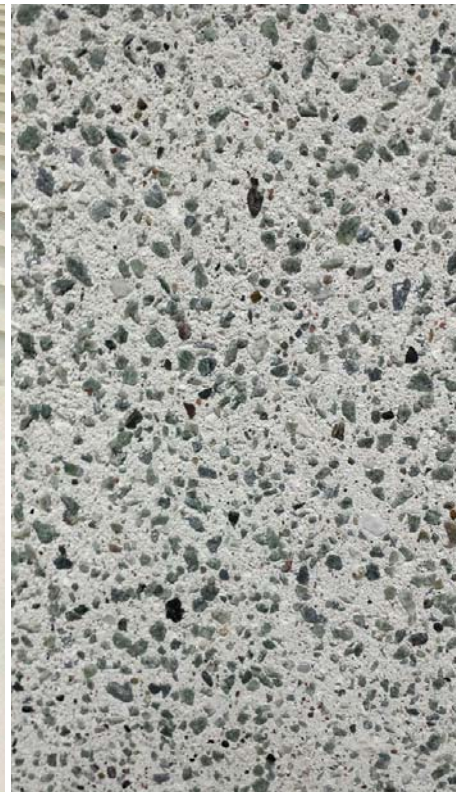
Wash-out surface providing a more exclusive look with blue and green aggregates.
